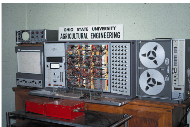
Figure 4. Electronic analog computer simulation of the laser-beam automatic grade-control system on the plow.
