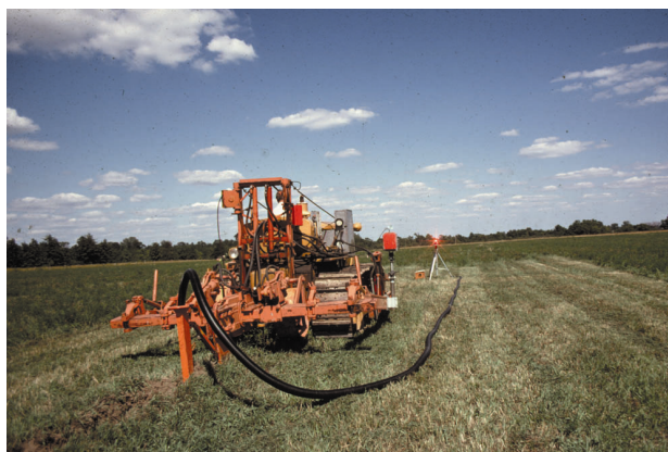
Figure 1. USDA-ARS prototype draintube plow with laser-beam automatic grade-control system.
