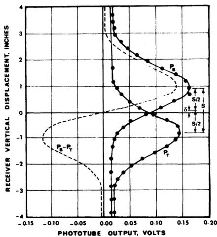
FIG. 3 Variation of phototube outputs with vertical displacement.
