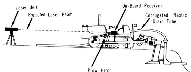
FIG. 1 Schematic of the laser beam automatic depth and grade control system for a draitube plow.
