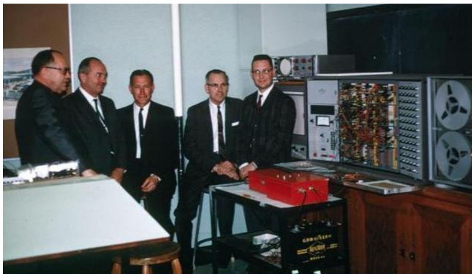
Fig. 11 – Analog Computer Simulation setup to evaluate the Laser-Beam Depth & Grade-Control Circuits. Observers: (L to R) 5 ; C. Wadleigh, W. Raney, R. Stewart, G. Schwab, with J. Fouss; (missing from the photo is M. Hamdy, an adviser to Fouss on the analog simulation project.) The dimension “S” shown in Fig. 12 is the vertical distance between the top and bottom rows of
