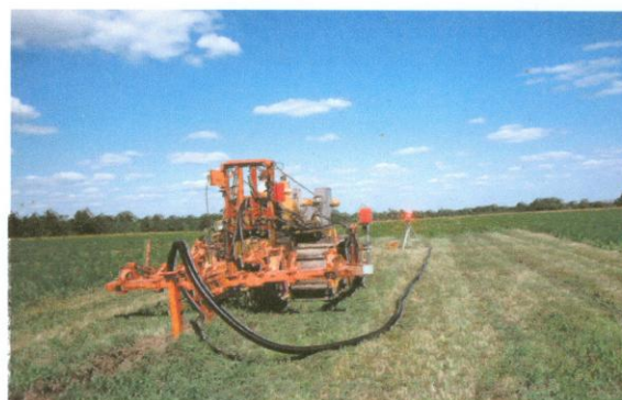
Figure 1. USDA-ARS prototype draintube plow with laser-beam automatic grade-control system.
