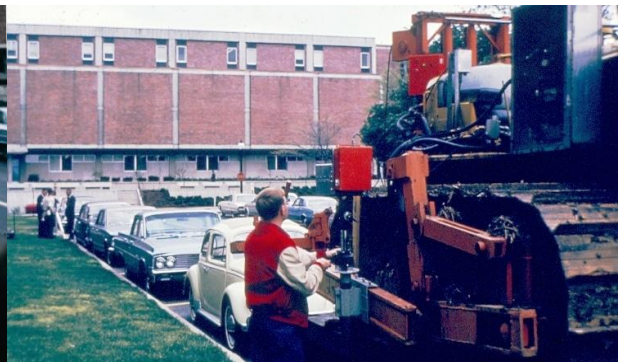
Fig. 10a – Laser-Beam Projector at 50 m away. Fig. 10b – Laser-Beam Received on Plow Beam.
