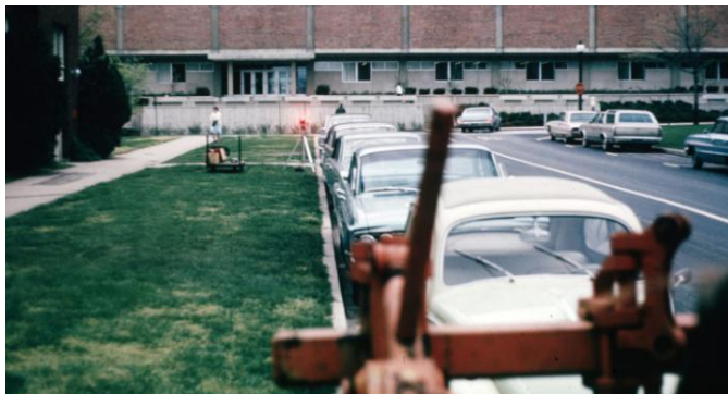
Fig. 10a – Laser-Beam Projector at 50 m away. Fig. 10b – Laser-Beam Received on Plow Beam.
