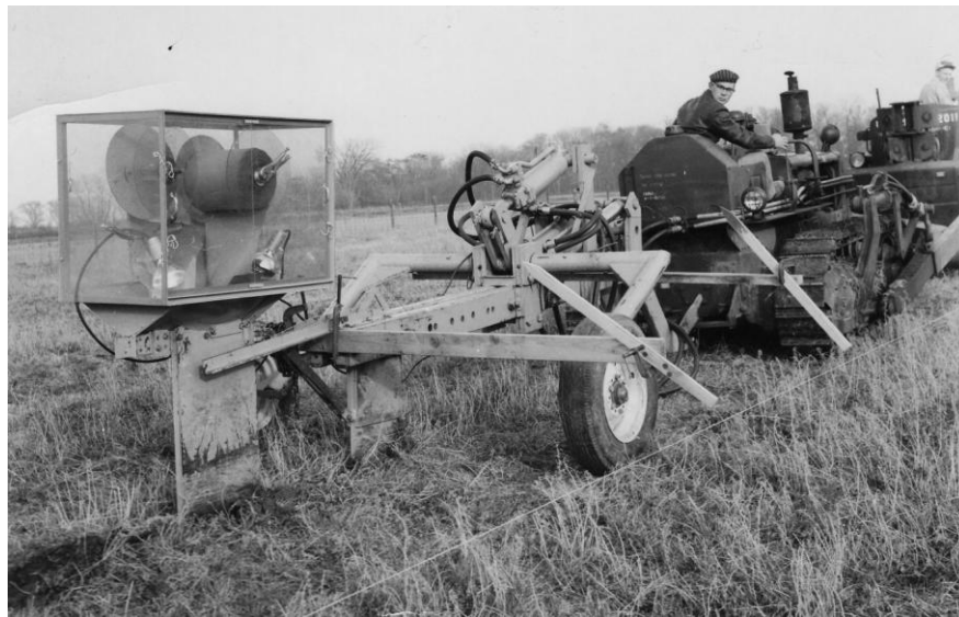
Fig. 2. Floating-Beam Mole-Drain Plow equipped with a “zippered” plastic mole-drain liner installation attachment; wheels on plow frame were for transport only when out of the ground, not plow depth control.
