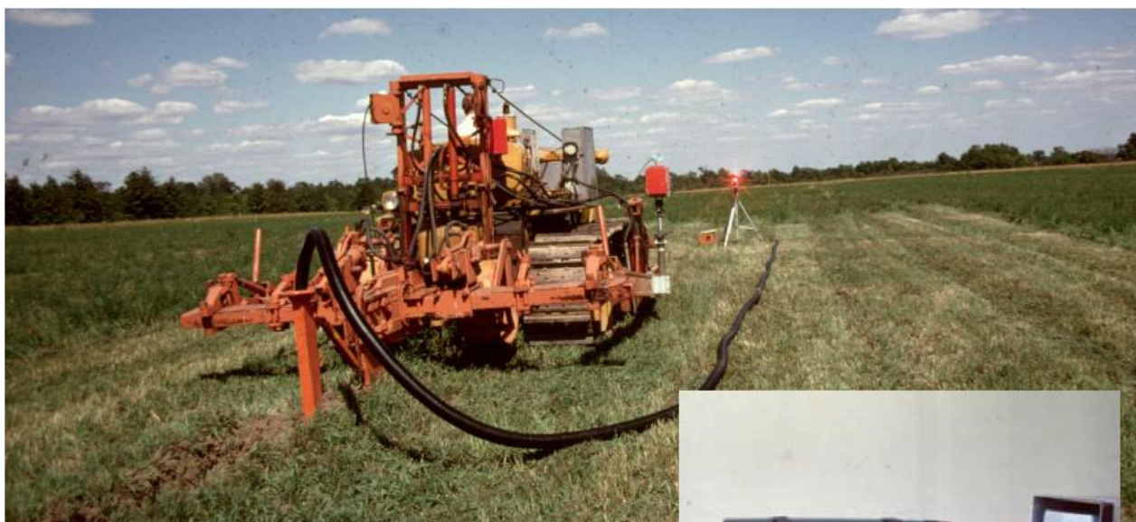
Figure 1A (above) Research prototype laser-controlled drainage plow. 1B. (inset) Laser transmitter with shielding removed to show telescope and chopper blade.
