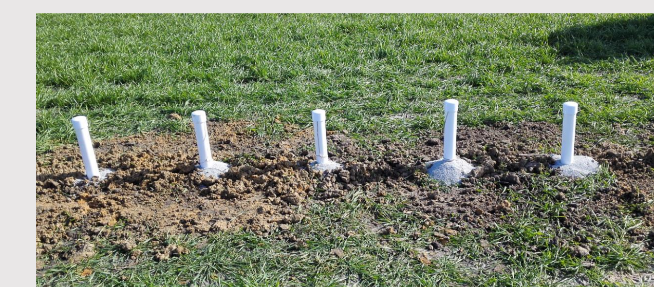
Water table and water quality wells
