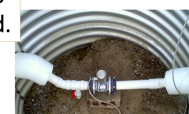
Flowmeter takes drain flow measurements every hour.
