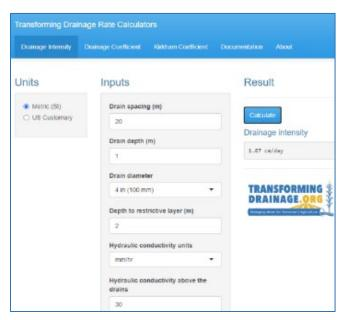
User interface for the Drainage Rate Calculator. Users can determine three standard coefficients for characterizing the hydraulics of subsurface drainage systems.
