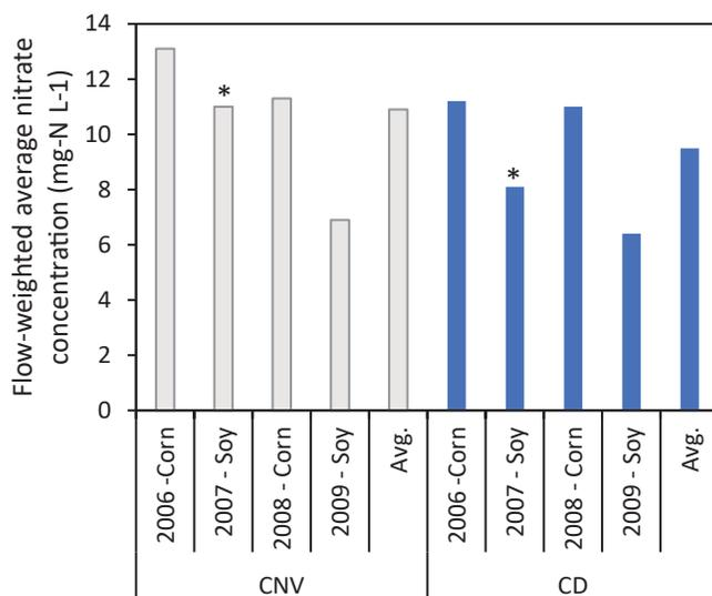
Figure 2 Flow-weighted average nitrate concentration for conventional (CNV) and controlled drainage (CD) for the years 2006 – 2009 and the average over all years.
