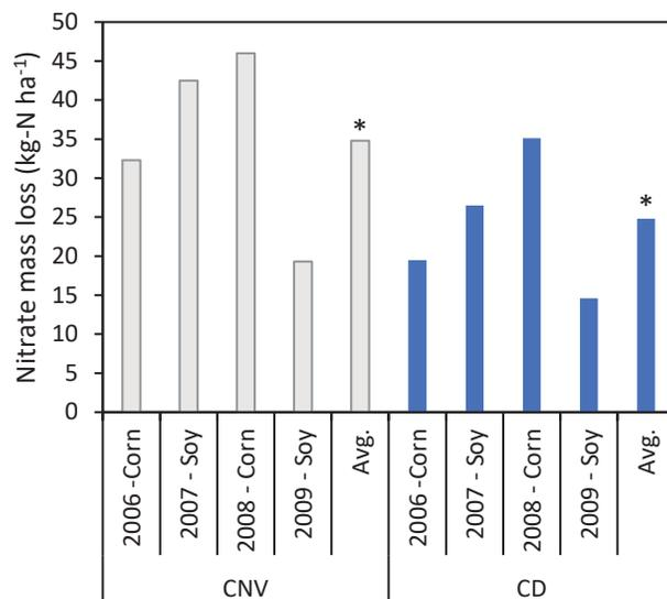
Figure 3 Nitrate mass loss for conventional (CNV) and controlled drainage (CD) for the years 2006 – 2009 and the average over all years.
