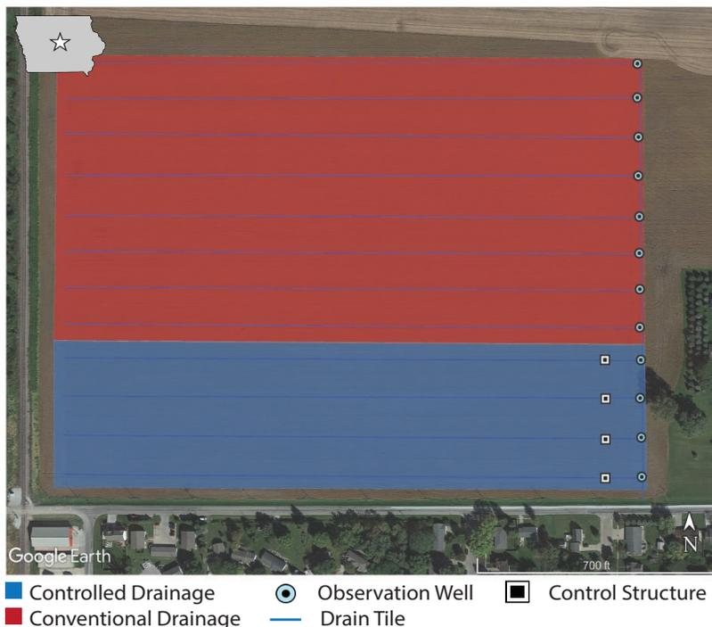
Figure 1. Drainage map of Story County, Iowa drainage research site.
