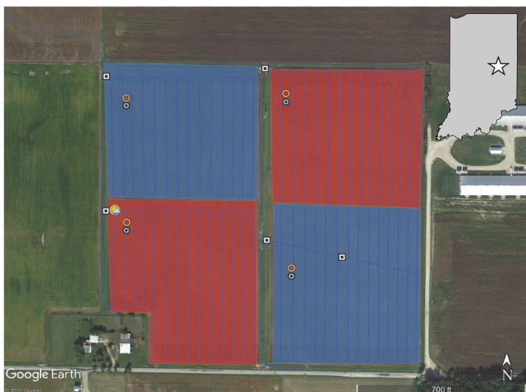
■ Controlled Drainage ■ Conventional Drainage — Drain Tile Control Structure ● Observation Well ○ Soil Moisture Sensor ☀ Weather Station
