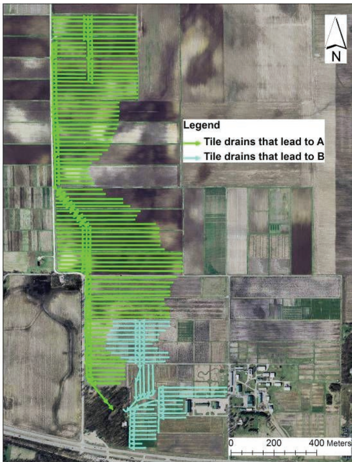
Figure 3. Map of tile drainage network at IN-TIPPECANOE.
